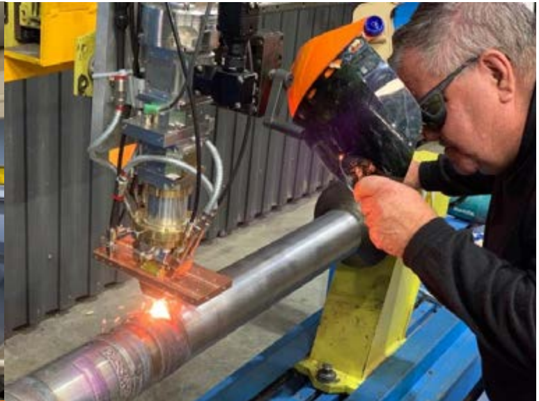
Laserline LDF diode laser for cladding at QSP Engineering, Brisbane QLD
